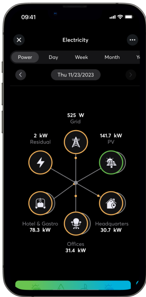
The Energy Flow Monitor in the Loxone App
