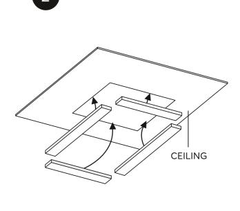
Cut a hole into the drywall (same measurement as the Back box) And fix 4 battens for mounting
