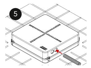
Connect the cable conduit. (Take care to avoid large gaps between back box and conduit)
