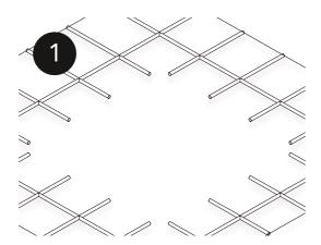
Determine desired location on the concrete formwork and cut out the steel reinforcement
