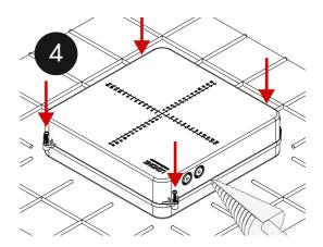
Attach the upper part of the box with the 4x screws. Use a step drill to cut out the holes for the cable conduit
